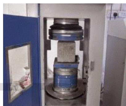
Fig.3.Compressive Strength test on Cube
